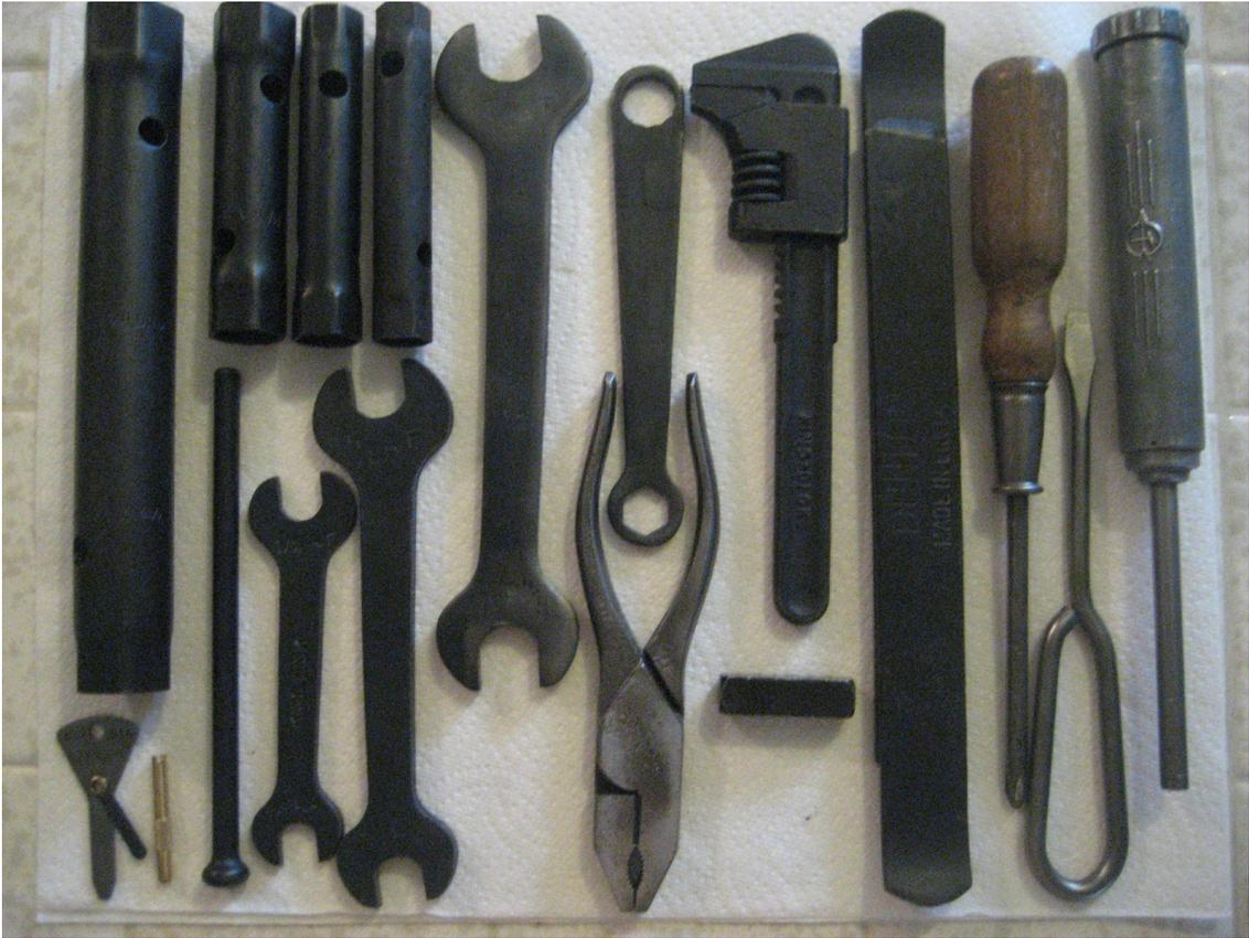
*Very original late MGA tool kit in excellent condition (the tools were not pitted). I still need to blacken the KING DICK pliers and bent wire screwdriver. C. Arndt*
